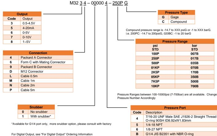
All Configurations are built with Voltage Reverse and Output Short-Circuit Protections.
